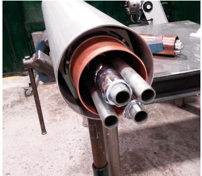
Figure 12: Production sample of a short transfer line running from the valve box to the cryo pump. Helium lines (top left and lower right tubes) are wrapped with superinsulation.
