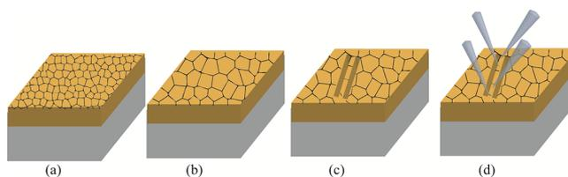
**Figure 3.** (a) Thin films are grown on (0001)-oriented  $\alpha\text{-Al}_2\text{O}_3$  substrates; (b) grain growth is obtained by an annealing treatment. (c) GBs are separated from their surrounding region by FIB milling, and the line is still connected at its ends to the film. (d) Four micromanipulators are used to probe the bicrystal electrical resistivity.
