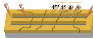
**Figure 4.** Schematic of a line containing several GBs within the thin film. Positions of the four needles used for the four-point measurement technique are demonstrated. Needles 1–3 are fixed at a specific position during the experiment, while needle 4 moves along the line from position 4 to 4''. Several GBs can be inspected within a single line.
