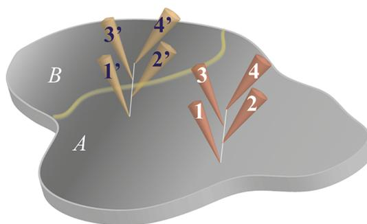
**Figure 6.** Schematic sketch illustrating the procedure to obtain GB resistivity by using the four-point-probe method. Single crystal resistivity is obtained for needles with positions 1 to 4; bicrystal resistivity can be deduced for needle positions 1' to 4'.
