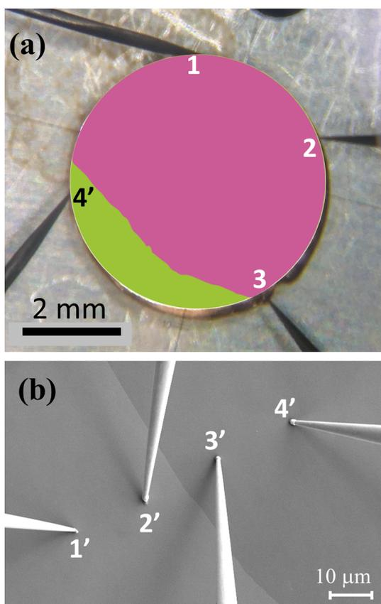
**Figure 9.** (a) van der Pauw contacts of the Cu bicrystal. The color code indicates the two grains based on SEM-EBSD measurement. (b) *In situ* four-point probe measurements across an individual GB in the bulk Cu.
