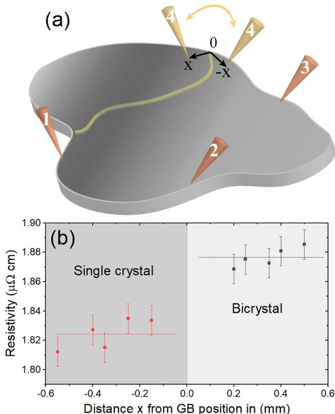
**Figure 5.** (a) Schematic of the van der Pauw method; needle positions 1 to 4 are applied for the resistivity measurements of a single grain of the bulk bicrystal, while positions 1 to 4' sense the bicrystal resistivity. Note that needles 1–3 are kept in the same position during the experiment, while needle 4 is relocated to 4'. (b) Resistivities of the single and bicrystal obtained with sub-mm changes in needle positions 4 or 4' near the GB.
