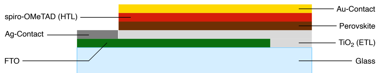
Figure 1.2. Schematic of the fundamental structure of a solar cell in n-i-p architecture.
