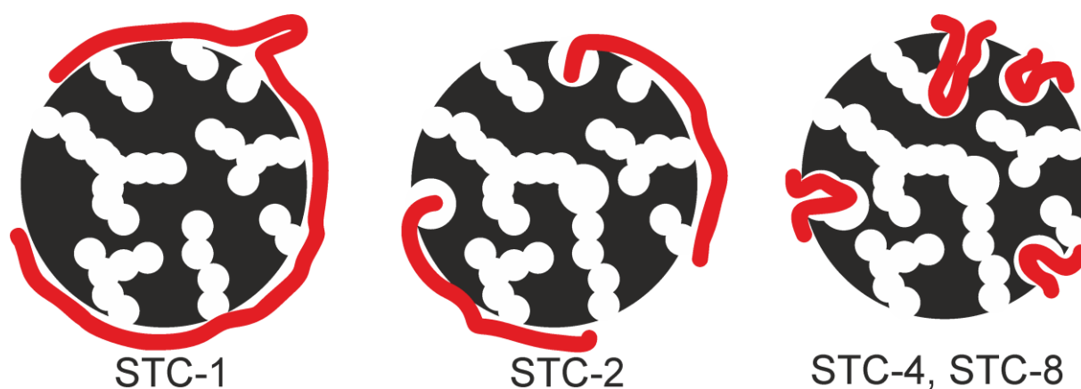
Figure 5.24. Proposed model of interaction between carbon (black), micropores (small holes), mesopores (big pores) and polymer (red)
