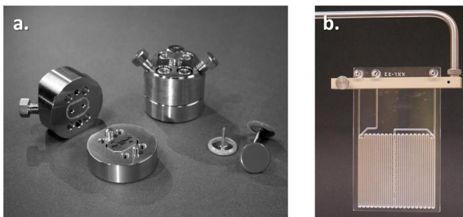
Figure 1.9: A typical microreactor. a. 4 way jet mixing device (left) and HPIMM (right) from Institut für Mikrotechnik Mainz (IMM) GmbH. b. Glass microreactor XXL from MERCK.
