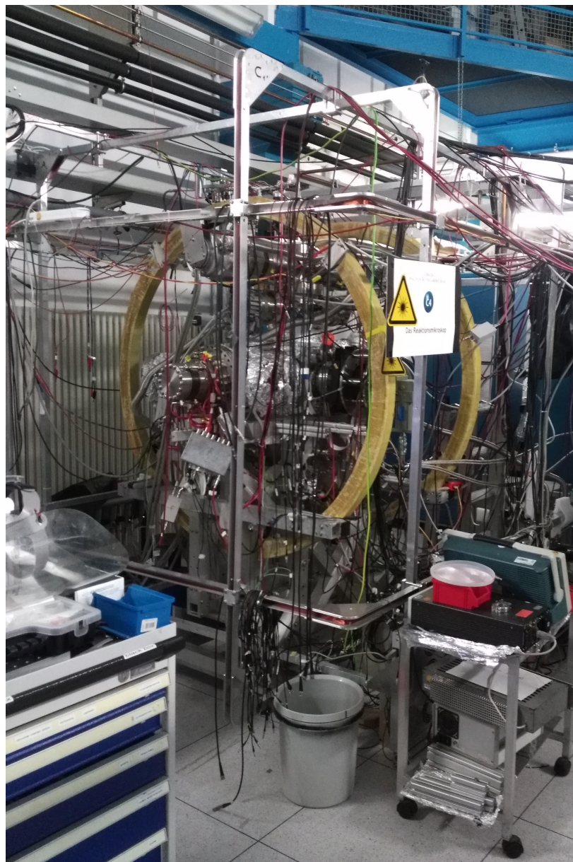
Figure A.1: Photo of the experimental set up. One can see the Helmholtz coils (Yellow isolation) and the square shaped coils to shade the earths magnetic field (In the metal profiles). In the middle of the coil arrangement, the vacuum chamber is located.
