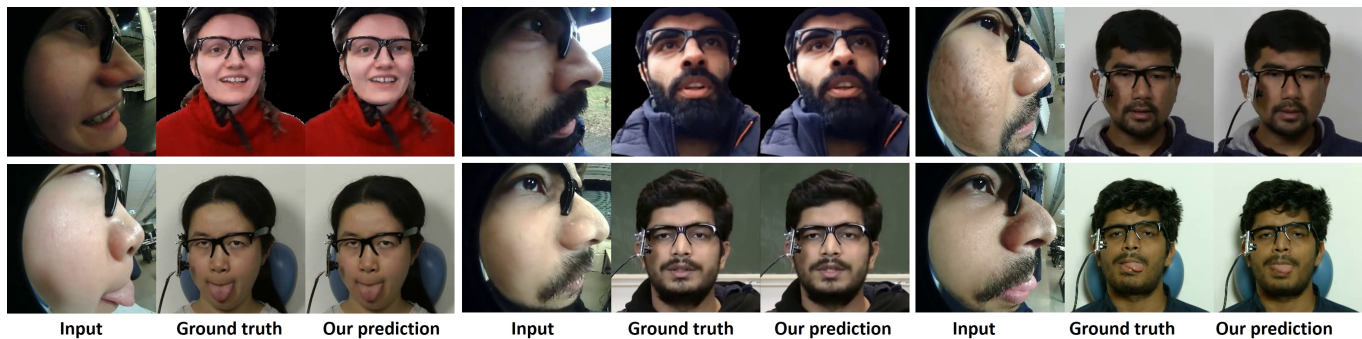
Fig. 1. We present an approach for hands-free videoconferencing. Given the view of an egocentric camera, that is attached to an eye-glasses frame, we predict a frontalised video stream which is common in videoconferencing.
