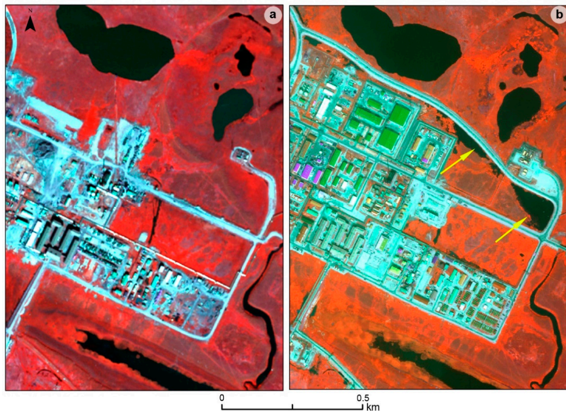
Figure 13. Color-infrared images (NIR-R-G) of infrastructure and thermokarst lakes in the Yamal Peninsula: Quickbird 02 acquired on 28 July 2004 (a) and GeoEye01 acquired on 18 July 2016 (b). The initiation of new thermokarst lakes is marked with yellow arrows in panel, which appeared after the construction of a concrete road.
