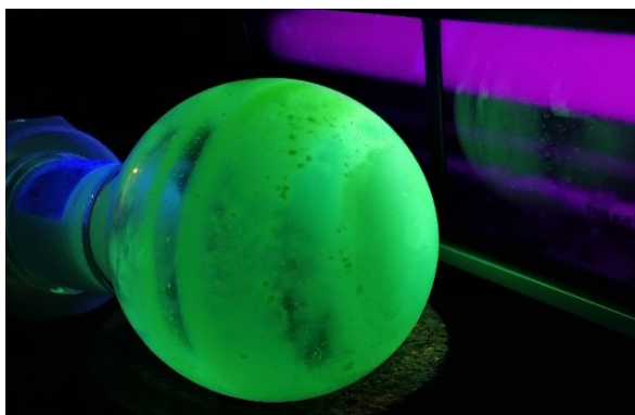
Figure 4.24: Photograph of the residue after Soxhlet extraction under UV irradiation at 356 nm.
