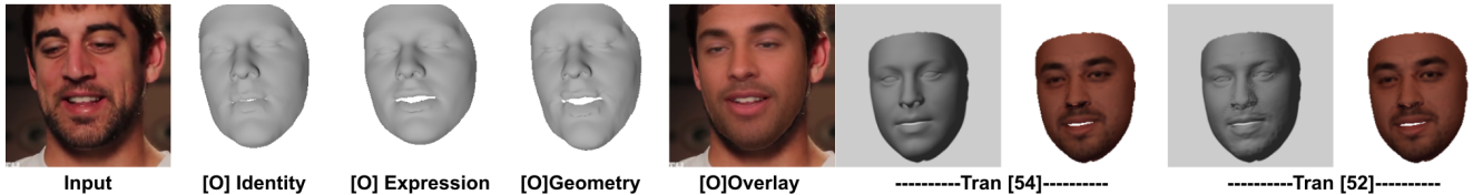
Figure 8. Both approaches of Tran et al. [56, 54] do not disentangle identity geometry from expressions. Our technique, however, estimates and disentangles all facial components. It also produces produces more accurate mouth shapes.
