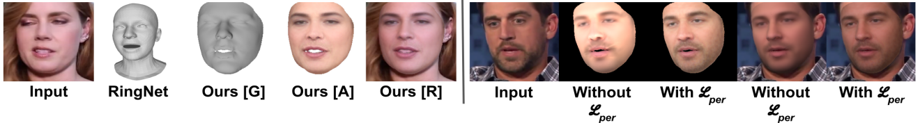
Figure 10. Left: Our technique better captures mouth shape and eye geometry than RingNet [44]. It also produces a photorealistic overlay. Right: Albedo and overlay is noticeably improved with perceptual loss \mathcal{L}_{per} (see 3rd and 5th column).
