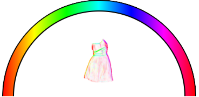
Figure I. Example of our garment structure visualization for one of the dresses shown in Fig. 1 from the main paper. We model the orientation as hue in HSV-color space, while each pixel’s saturation corresponds to the local gradient confidence.
