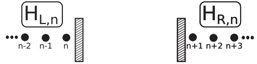
FIG. 1. Illustration of the semi-infinite Hamiltonians H_{R,n} (right) and H_{L,n} (left). The Hamiltonian H_{R,n} is obtained from the bulk Hamiltonian H_{\text{bulk}} by starting it at site m = n + 1 , whereas H_{L,n} is obtained by ending H_{\text{bulk}} at site m = n .
