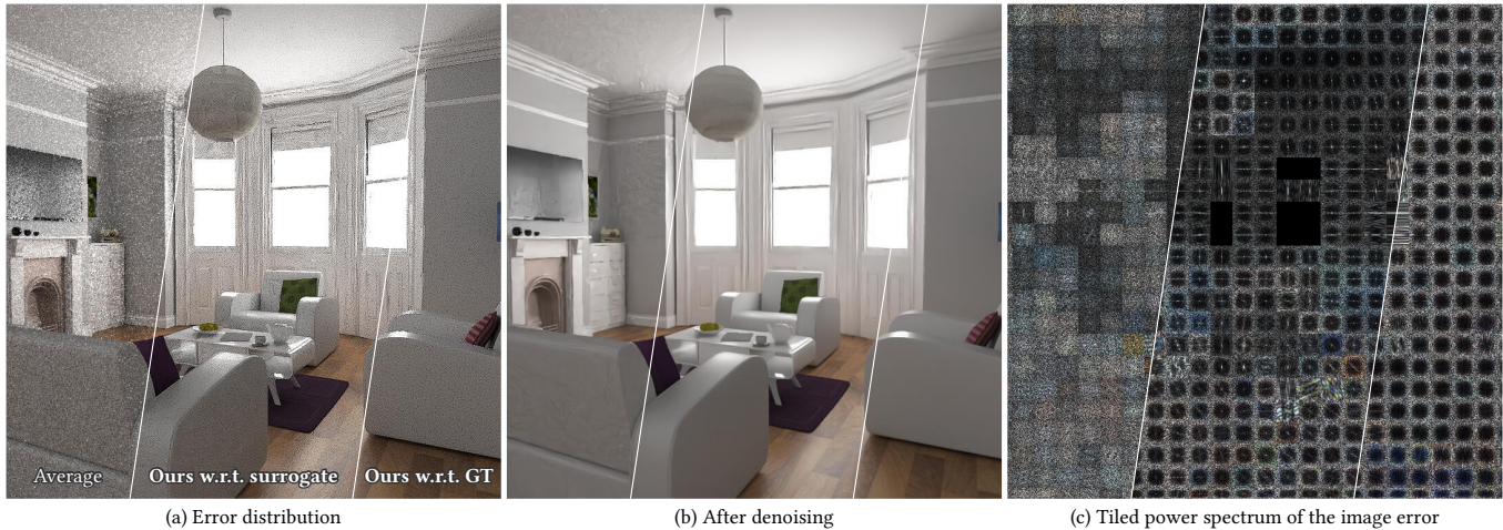
Fig. 1. Using our perception-motivated model, we analyze different ways to distribute screen-space error in Monte Carlo rendering, showing one such approach here. We start with a noisy image and some auxiliary data (surface normals and albedo). Average image (leftmost) is rendered with 16 samples per pixel (spp). Our method uses varying spp from the set: \{4, 8, 12, 16\} spp. (a) Our approach exhibits both visually pleasing screen-space error distribution (see Section 4.1 for details) while keeping less samples per pixel. Our energy model uses a guiding image, or surrogate , which can be created easily from the noisy estimate. We also show our method using the ground truth (GT) image as the guide. (b) To demonstrate the impact of error distribution on denoising, we apply Intel’s Open Image Denoiser [int 2018] on the images in (a): the white-noise distribution results in conspicuous artifacts, which are avoided when the error has a blue-noise distribution (as in our results). (c) The corresponding tiled power spectrum ( 32 \times 32 pixels per tile) of the error images from (a), confirming that our approach distributes error with a locally blue-noise spectrum.
