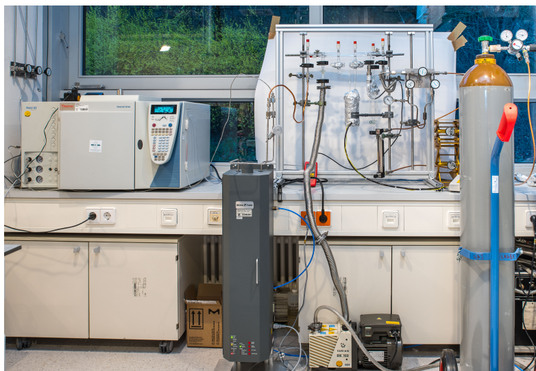
Figure 25: Picture of the experimental set-up. The gas-chromatograph on the left side, the getter and roughing pump on the bottom, below the chromatographic system. On the right hand side, the bottle supplying the helium is shown (credit: R. Lackner).
