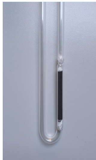
Figure 27: Picture of an exemplary column. Here filled with activated carbon. The adsorbent is fixed with glass-wool, so that the powder stays in place while carrier gas is flushed through the column.
