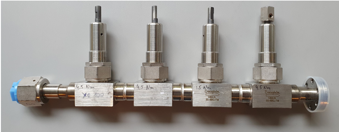
Figure 12: Xenon sample pipette. The port on the right is connected to the RGMS input port, the port on the left is used for baking, pumping and sample filling.
