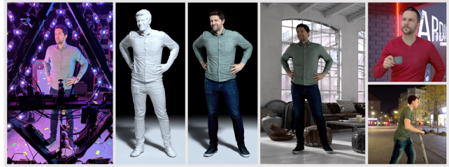
Figure 7: The Relightables system by Guo et al. [GLD*19] for free viewpoint capture of humans with realistic re-lighting. From left to right: a performer captured in the Lightstage, the estimated geometry and albedo maps, examples of relightable volumetric videos. Images taken from Guo et al. [GLD*19].
