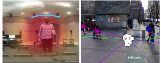
Figure 3. Including correct and coherent auditory information to the environment has been proved to increase realism and immersion. Left: A system that automatically generates ambisonic information that creates a smoother acoustic information for the scene [116]. Right: A framework to include auditory information into 360° panoramas depending on the elements that conform the scene [66]. In both cases, their validation experiments yield users' preference when auditory information is included, and an overall increase in the perceived realism and immersion in the virtual experience.
