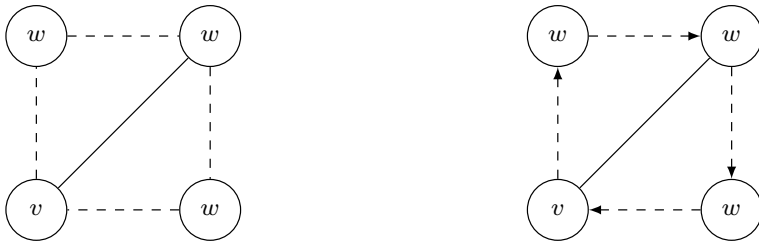
Fig. 8 A Hamiltonian cycle (dashed, left) can directly be translated to a feasible walk (dashed, right) through all waypoints
