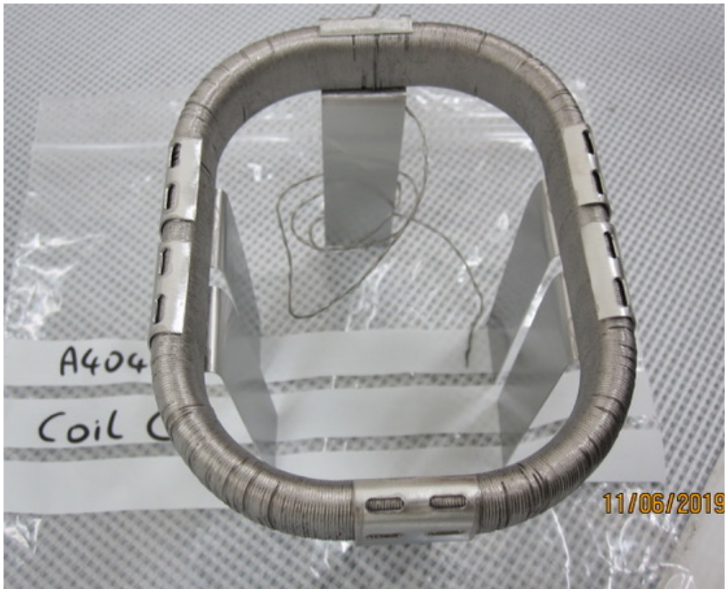
Figure 3: Rogowski coil prototype for the ITER divertor cassette
