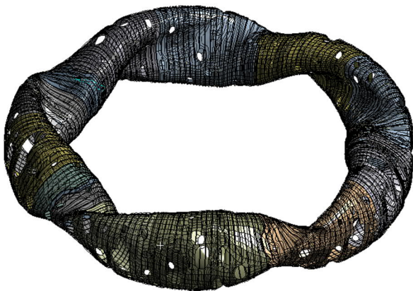
Fig. 2. The shell-beam model of the PV
