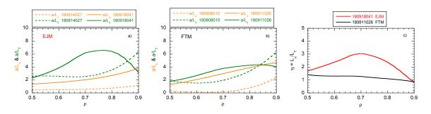
**Figure 8.** Normalised density gradient (in orange) and temperature gradient (in green) for gas fuelled (broken lines) and post-pellet plasmas (solid lines), in the standard EJM (a) and in the high iota FTM (b) configurations. (c): ratio of the temperature gradient and the density gradient for post-pellet plasmas in the standard (in red) and high iota (in black) configurations.
