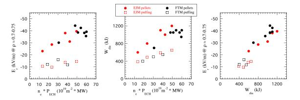
Figure 2. Local  $E_r$  intensity measured by DR at  $\rho \sim 0.7$ -0.75 (left) and diamagnetic energy (centre) during the post-pellet high confinement phase (solid symbols) and in gas fuelled plasmas (open symbols) as a function of the product  $n_e \times P_{ECH}$ . The relation between the  $E_r$  intensity and the diamagnetic energy is shown in the right panel. Standard magnetic configuration EJM is represented in red and high iota configuration FTM in black.
