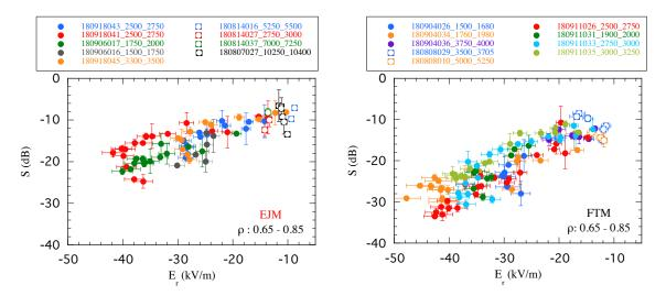
Figure 7. Density fluctuation level as a function of local  $E_r$  measured within the radial range  $\rho = 0.65 - 0.85$  in several experimental programs in the standard (left) and high iota (right) magnetic configurations. Solid symbols represent data obtained during the post-pellet phase and open symbols in gas fuelled reference programs.
