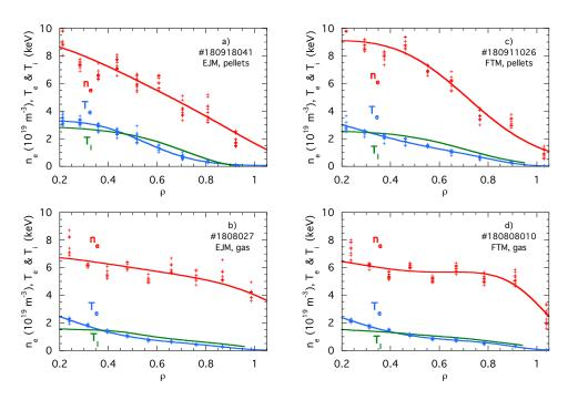
Figure 3. Electron density and temperature profiles measured by Thomson Scattering diagnostic and ion temperature profile measured by XICS diagnostic during the postpellet phase in the standard EJM (a) and high iota FTM magnetic configuration (c), and in the reference gas fuelled plasmas in the two configurations (b) and (d), respectively. The solid lines represent the fits to the experimental values (symbols) measured during the time interval of the DR analysis.
