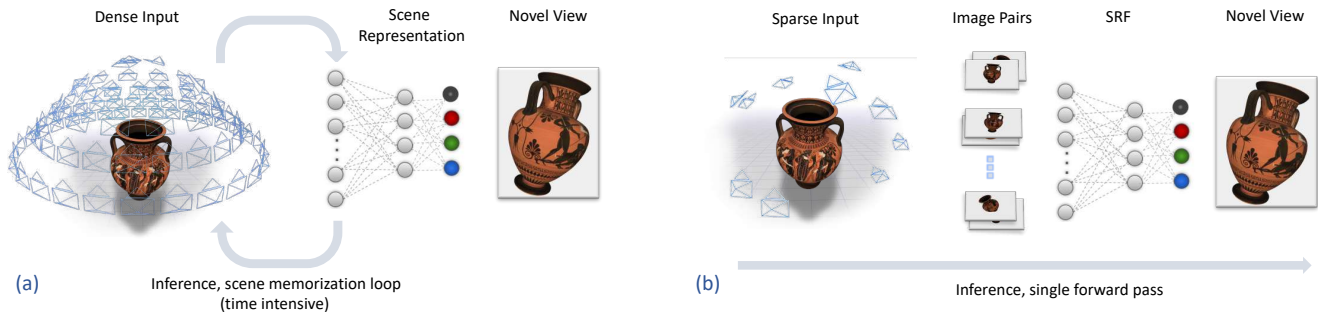
Figure 2. Pure data-driven view synthesis and SRF (ours) . Existing methods achieve remarkable realism representing scenes with a neural network. A model is trained specifically for a scene to synthesize high-quality novel views. However, this requires dense views and 2 days of training per scene. In this work, we address the more challenging task of novel view synthesis from sparse and spread-out views, using a single forward pass through the network, to instantly obtain the result.
