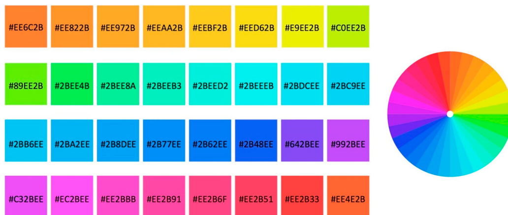
Figure 1. The game's colour space. Each colour is given its associated Hex code (as used by the app). Each of the game's 32 colours is drawn from the CIE2000 colour space (see Luo et al., 2001), in constant perceptual distance to its left and right neighbours. This includes the first and last colour, meaning that the space is circular and can be represented as on the right. Figure adapted with permission from Morin et al. (2020).
