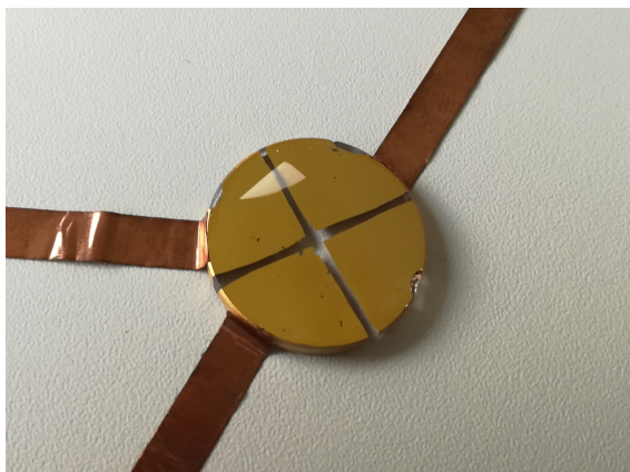
Figure 4.3: Electrochemical cell geometry for heterodyned potential-dependent SFG measurements. For clarity the window, that is attached via parafilm and is slightly tilted through the Teflon wedge, is not shown.
