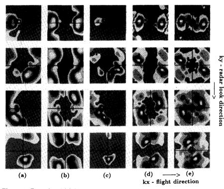
Figure 1: Examples of (a) first-guess wave spectra, (b) simulated first-guess SAR spectra calculated from (a), (c) optimally fitted wave spectra, (d) optimally simulated SAR image spectra calculated from (c), and (e) ERS-1 SAR wave mode image spectra obtained on Sept. 11, 1992. The normalized spectra are plotted in linear scale with a color-coded isoline spacing of 0.1. Here  $k_x$  and  $k_y$  are the wavenumber components in azimuth (flight) and ground range direction, respectively.
