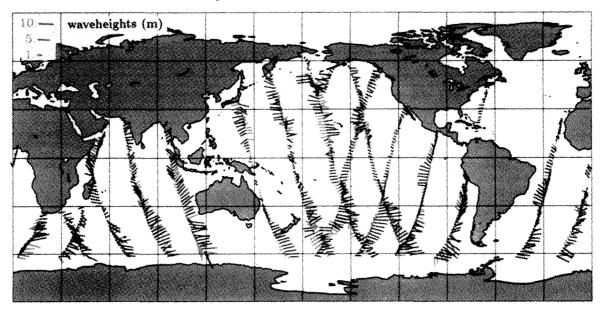
Figure 3a: Significant wave heights (in log. scale) and main propagation directions of the principal wave components obtained on Sept. 11, 1992 extracted from ERS-1 SAR wave mode image spectra.
