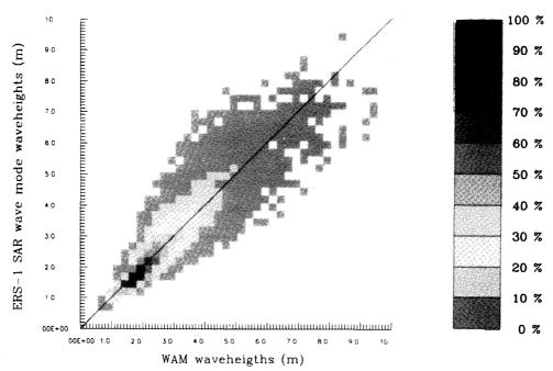
Figure 2a: Global comparison of significant wave heights computed with ECMWF WAM wave model and extracted from ERS-1 SAR wave mode image spectra, respectively, obtained during the period from Sept. 1 - 30, 1992 (15668 entries). The number of entries of individual boxes  $(0.25 \text{ m} \times 0.25 \text{ m})$  are color-coded. Each color represents 10% of the data.
