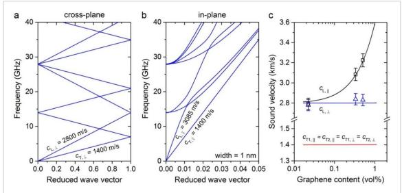
**Figure 4.** Calculated phononic band structure and effective sound velocities in Gr/PMMA Bragg stacks. The phononic band structures of Gr(3.3)/PMMA in the (a) cross-plane and (b) in-plane directions. The effective sound velocities of the lowest longitudinal and transverse branches in the long wavelength limit are indicated. (c) The effective longitudinal (L) and transverse Gr/PMMA stacks as a function of the graphene volume fraction.
