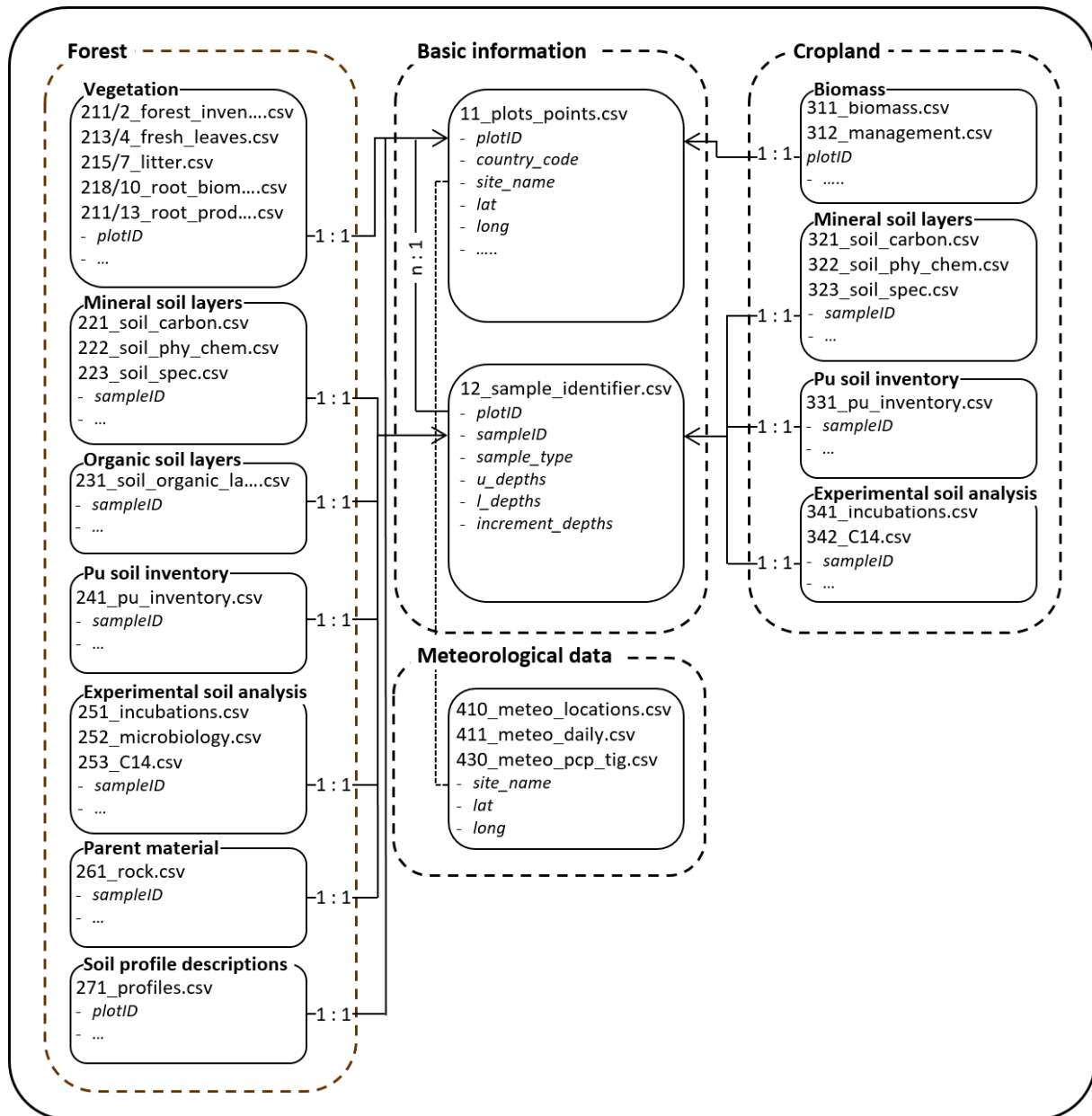
Figure 6. Overview of linkages between datasets in the TropSOC database v1.0. Note that for each data .csv file a .pdf file is given detailing the metadata of the respective data sheet.
