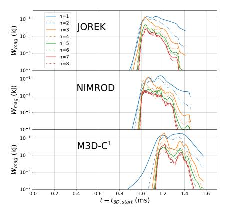
Figure 5: Magnetic energies from the modes  $n \in [1, 8]$  in JOREK, NIMROD and M3D-C<sup>1</sup> over time.
