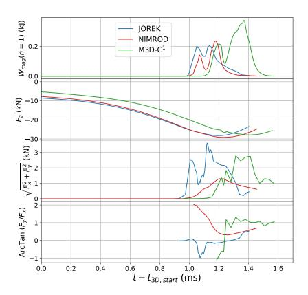
Figure 7: Time traces of the n=1 magnetic energy, the vertical force, the total horizontal force and the toroidal phase of the total horizontal force.
