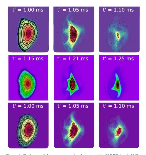
Figure 6: Evolution of the pressure at the plane  $\phi=0$  in JOREK (top), M3D-C<sup>1</sup> (middle) and NIMROD (bottom) in arbitrary units. The pressure plots are overlaid with corresponding Poincare plots showing the magnetic field topology.
