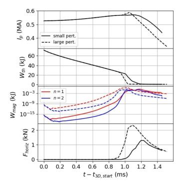
Figure 13: Comparison of plasma current, thermal energy, magnetic perturbation energy, and horizontal force from NIMROD computations with perturbations at the start of the 3D phase differing by 1000 in amplitude. The small-perturbation case is the one described in preceding sections.
