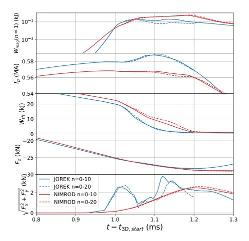
Figure 10: Magnetic energy of the n=1 mode, plasma current, thermal energy, vertical and horizontal force for two JOREK and NIMROD runs with different number of toroidal harmonics. The NIMROD computations shown here have been run with 2D resistivity and increased parallel viscosity—see the text.
