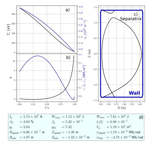
Figure 1: Equilibrium used as initial condition for the benchmark. (a) Temperature and density profiles, (b) safety factor profile and poloidally averaged toroidal current density profile  $(\oint_{\psi=\text{const}} J_{\phi} dl/\oint_{\psi=\text{const}} dl)$  as functions of the normalized poloidal flux. (c) Wall and initial separatrix geometry. (d) List of relevant scalars describing the equilibrium.
