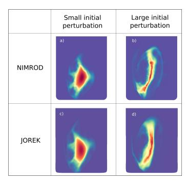
Figure 14: Comparison of pressures from NIMROD and JOREK computations with small-amplitude (a,c) and large-amplitude (b,d)  $n \geq 1$  perturbations, just prior to initial saturation of the (2,1) mode in each case. The plots display the  $\phi=0$  plane except for figure (d) where  $\phi=1.12\pi$  was chosen to compare the 3D plasma state in the same phase.
