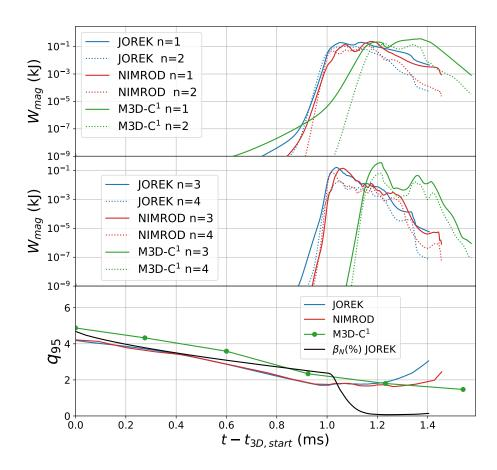
Figure 3: Magnetic energy of the toroidal harmonics  $n \in [1, 4]$  in the three codes as a function of time. The time traces of the edge safety factor  $(q_{95})$  and the normalized  $\beta_N$  in JOREK (black curve) are also shown in the bottom figure.
