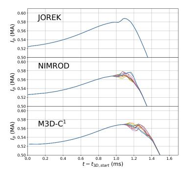
Figure 9: Total toroidal current  $(I_p)$  computed at 10 equidistant poloidal planes with  $\phi = 2\pi k/10$  and k = 0, 1...9 in JOREK, NIMROD and M3D-C<sup>1</sup>. Note that for JOREK the curves are indistinguishable and no toroidal current asymmetry is found.
