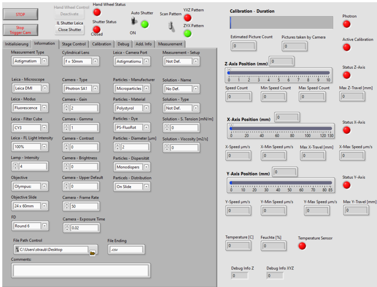
Figure A.4.: Graphical user interface of the written control software. The inner tabular structure offers different control options. The other data is, independent of the chosen tab, always visible.
