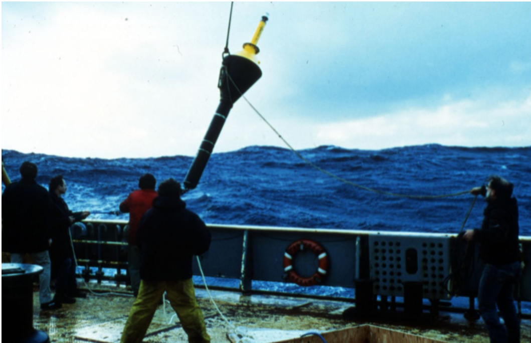
Figure 6 - Deployment of Metocean 7147 buoy in the Pacific Ocean, 1988. Image located in Supplementary Information Files for art. no. 1990.0017. Ingenium: Canada’s Museums of Science and Innovation, Ottawa.
