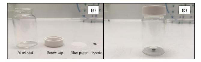
**Figure 5**: Experimental setup for fumigation toxicity assay. (a) Materials used in the experiment, (b) the complete setup of the experiment where a single beetle is placed at the bottom of the glass vials and the filter paper containing test chemical was secured on the top under the lid.
