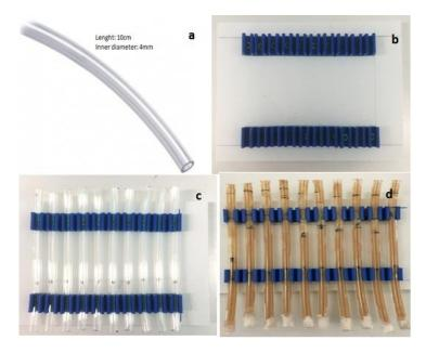
**Figure 6**: Bark beetle feeding assay apparatus: (a) pneumatic tube, (b) a wooden board to attach the tubes, (c) the tubes attached to the board and numbered, (d) beetles feeding on an artificial diet mixed with different monoterpenes.
