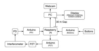
FIG. 5. Signal flow chart for the exhibit. A Raspberry PI runs the exhibit software and interfaces with the piezo-electric transducers (PZTs) and the photodiode (PD). When used at the Thinktank Birmingham Science Museum, the PC is separated by 30 m from the rest of the exhibit, so communication must be be done via ethernet rather than a simpler, faster USB connection (USB is limited to 5 m).
