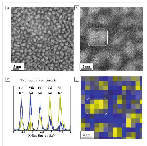
Figure 1. (a, b) HAADF-STEM images of as-deposited CSS thin film showing two distinct features: islands (bright) and continuous layer (dark). (c) Two major spectral components of EDS spectrum imaging and (d) their spatial distribution in corresponding colors (islands in yellow, continuous layer in blue). The islands contain more Co and Ni. the continuous laver is enriched in Cr. Mn. and Fe.
