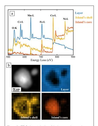
Figure 5. EELS characterization of the layer, one large and one small island. An oxide shell is surrounding the islands after the heating experiment. (a) EELS spectra of the three spectral components. (b) HAADF STEM image and color-coded mapping of the three spectral components showing their distribution (layer = blue, island's shell=yellow, island's core=orange).
