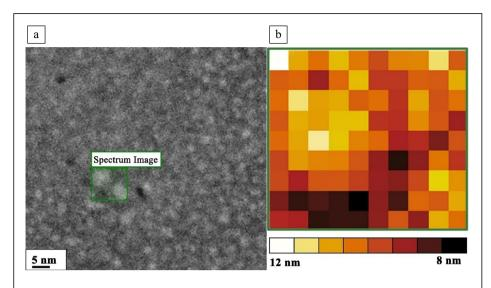
**Figure 2.** (a) STEM-HAADF image of the film after sputtering (initial state) where the region for the EELS characterization is marked. (b) EELS thickness map showing that the continuous layer and islands have different thicknesses.
