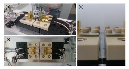
**Figure S2:** Photographs of the stretching setup. (a) Setup with light microscope above the sample. (b) Stretching setup top view. (c) Pre-stretched composite sample.
