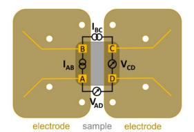
**Figure S3:** Sketch of the two electrodes and their respective electrical contacts (A, B, C, D). The composite sample is depicted in grey. The input currents (AB/AD) and the voltage drop (CD/BC) of the Van der Pauw measurement are shown.
