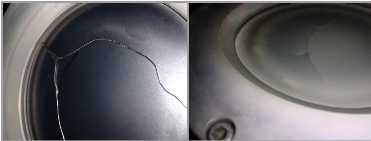
Figure 4.3: Photo of two different targets mounted in the reactor. Both broke after a process. One gray, metallic target is shown on the left. On the right side one white target is shown. After a few depositions this target has partially turned gray.
