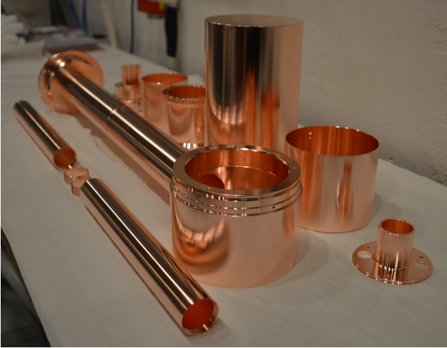
Figure 5: Electropolished copper cryostat parts used for the construction of the first CONUS detector C1.
