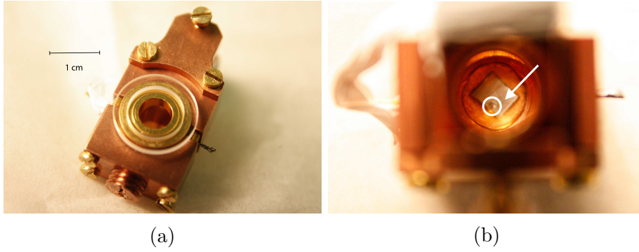
Figure 5.13: (a) An image of the assembled beryllium target and optics along with (b) a close-up view where the previously ablated region is visible.
