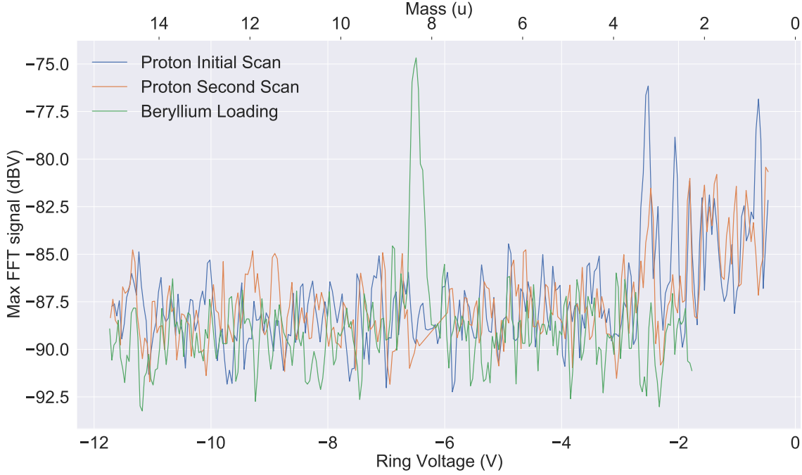
Figure 6.1: Three mass spectra taken in the ST are shown. Typically beryllium ions are loaded at lower pulse energies than protons. The measurement shown here was intended to find the transition point between optimal beryllium loading energy and optimal proton loading energy. In the ST, this configuration is optimized for the beryllium ions although, as seen in the second x-axis, the different voltage supply configuration introduces offsets in the ring voltage (and thus mass). The beryllium ions appear as a large, clean peak while the proton peak is smeared out and decays with successive scans in which high energy particles escape the trap at low voltages.
