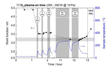
**FIGURE 2.** Influence of hydrogen plasma pulses on the surface work function of the C12A7:e<sup>-</sup> sample. The recorded sample surface temperature is additionally plotted (no active heating applied).
