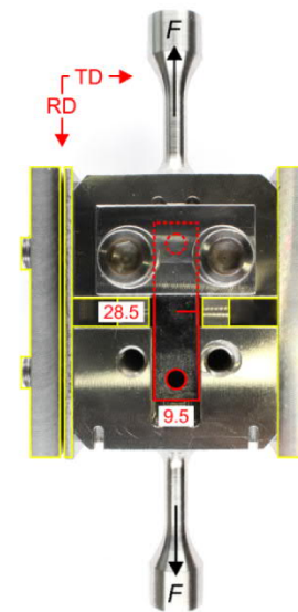
Fig. 1. Specimen, specimen fixture, and assembly device. Specimen geometry and outer specimen dimensions are highlighted in red. The thickness of the specimens varies and is equal to the thickness of the respective sheet. Furthermore, the alignment of the rolling direction (RD) and transverse direction (TD) with respect to the notch position is provided. Components of the assembly device are bordered in yellow. A detailed sketch of the experimental setup is given in an earlier publication [7]. (For interpretation of the references to color in this figure legend, the reader is referred to the web version of this article.)
