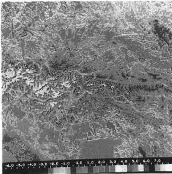
Figure 6 - a) \Delta T_4' for the daytime overpass in steps of 0.5 K indicated by different colours (see scale below image); b) \Delta T(x,y) + \Delta T_4' for the same scene.
