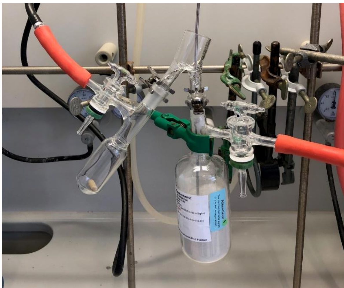
Figure S1. Use of “Argon pants”. The reaction flask and reagent flask are connected via a glassware with two legs and an open top. Argon is run through both Schlenk flasks continuously during operation, ensuring an inert atmosphere and allowing weighing of air-sensitive compounds like \text{Ni}(\text{cod})_2 without use of a glovebox. Note: compound shown in picture is not \text{Ni}(\text{cod})_2 .
