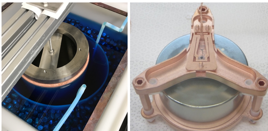
FIG. 8. Left: Cu electroforming bath running underground at SURF. Right: LMFE electronics board attached to four pico-coax cables, held in an EFCu spring clip affixed to a MAJORANA DEMONSTRATOR Ge-detector mount.
