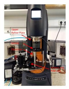
Figure 30: The assembly of in situ microscopy unit to the DHR-3 Rheometer.
