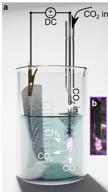
Figure 9.4: DC Plasma generation in aqueous electrolyte. (a) The DC-plasma electrode is covered by a glass pipette, except for the protruding Pt tip. CO 2 gas is flown through the pipette directly into the plasma. A Pt-mesh is used as a counter electrode. (b) Photo of the plasma electrode in operation.
