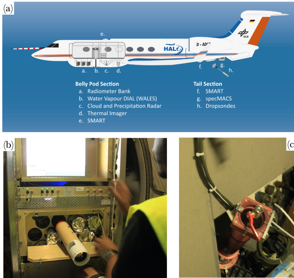
Figure 2.2: (a) Figure from Stevens et al. (2019a), showing the setup of instruments aboard HALO for the NARVAL2 and EUREC 4 A field campaigns, in addition to HALO’s default configuration. The thermal imager was available only for EUREC 4 A. (b) Photograph taken during a dropsonde’s initialisation a few minutes before its launch. The unpacked dropsonde is connected to the AVAPS computer whose screen is seen above the dropsonde rack and (c) Photograph of the pneumatic launch-chute located on the starboard side of HALO, oriented downwards and facing away from the fuselage. Photographs (b) and (c) were taken during EUREC 4 A flight HALO-126 and are from Konow et al. (2021).
