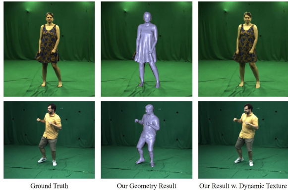
Fig. 8. Our geometry and texture networks generalize well to unseen motions as the geometry overlays nicely onto the ground truth frame and the final textured result looks almost identical to the ground truth. Importantly, our method does not take the ground truth frame as an input as it only takes the unseen motion from the video.
