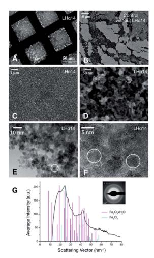
Fig. 2 (A) TEM image of LH $\alpha$ 14-templated iron oxide nanosheets spanning the holes of a TEM grid. (B) SEM image of iron oxide film precipitated without peptides and deposited onto a silicon wafer. (C and D) SEM images of LH $\alpha$ 14-precipated sheets. (E) TEM image of freestanding nanosheets. The higher resolution TEM in (F) shows crystalline domains. (G) Electron diffraction pattern of the nanosheets.
