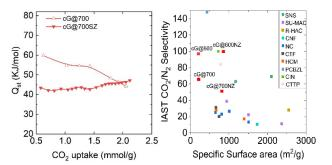
**Figure 5.** (Left) CO<sub>2</sub> heat of adsorption against CO<sub>2</sub> uptake of samples derived from guanine at 700°C and (right) a plot showing the CO<sub>2</sub>/N<sub>2</sub> IAST selectivity of guanine condensates compared within the state of the art of carbon based materials. Reproduced with permission from reference <sup>50</sup>.
