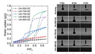
**Figure 6.** (Left) Isotherms showing record values of water adsorbed in carbonaceous materials derived from uric acid. (Right) Photographs showing the very fast adsorption of water in uric acid derived materials compared to Kuraray carbon. Reproduced with permission from reference <sup>52</sup>.
