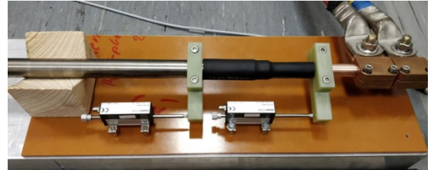
Fig.7: Termination of 3m sample with electrical connection and measuring devices
