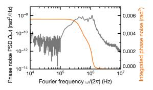
FIG. 4. Power spectral density (PSD) of the phase noise of the pump laser,  $\mathcal{L}(\omega)$ , relative to the ULE reference cavity. This was determined from the measured power spectral density of the PDH error signal. The PSD is shown in gray. The orange line corresponds to the integrated PSD, with the integration beginning at high frequencies.
