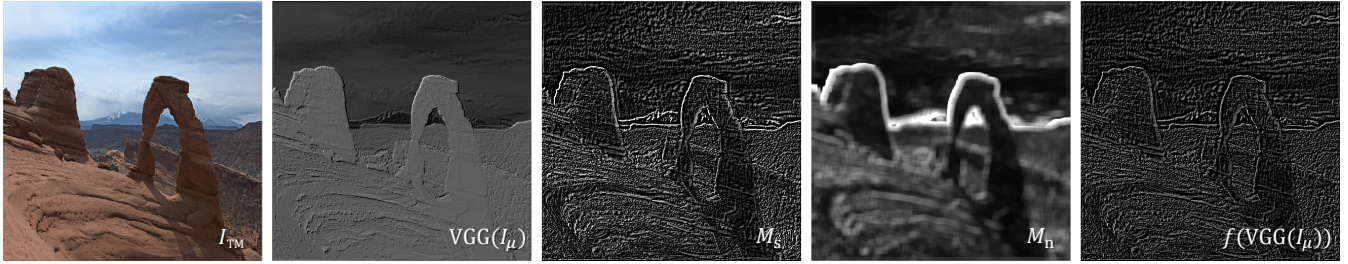
Figure 5: Feature contrast masking visualization of VGG feature maps (1st layer, 18th channel). From left to right: tone mapped image I_{TM} , original VGG feature map VGG(I_\mu) , and feature contrast self-masking M_s , neighborhood masking M_n , and final f(VGG(I_\mu)) masking terms.
